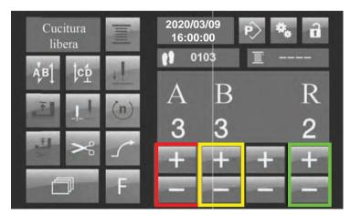
Fig.5 Free stitching interface - initial backtack settings.
