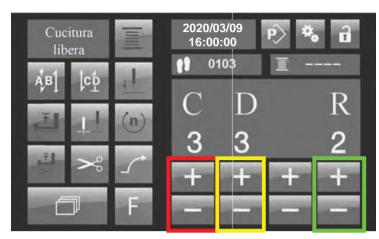
Fig.6 Final backtack interface.
