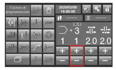
Fig.13 Programmed stitching interface, multi-stage switching.
