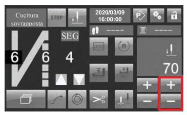
Fig.10 Overlapping stitching interface - fixed needle setting.
