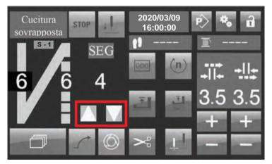
Fig.11 Overlapping stitching interface - Number of segments
