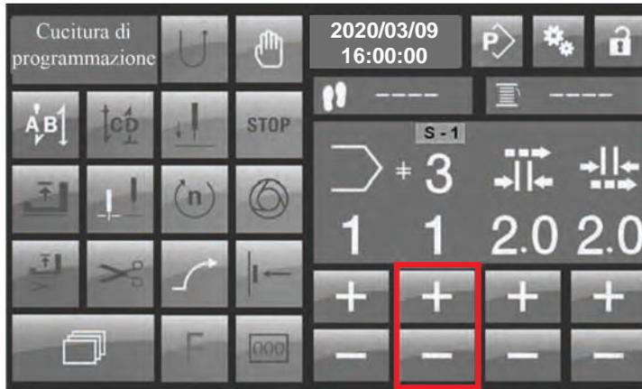
Fig.13 Programmed stitching interface, multi-stage switching.
