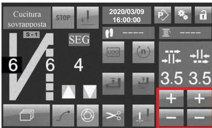
Fig.9 Overlapping stitching interface - wheel value setting.
