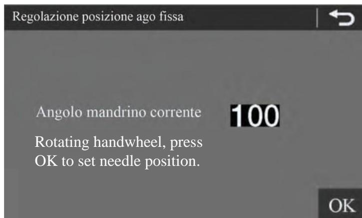
Fig.8 Free stitching interface - fixed needle position setting.
