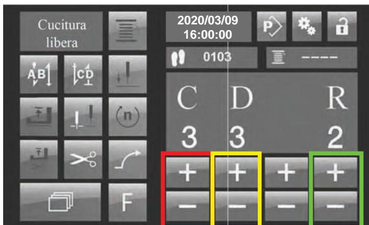
Fig.6 Final backtack interface.
